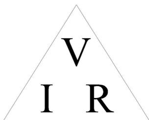
This is a representation of Ohms Law. It is shown this way to make it easier to arrange in order to find one of the missing variables.
